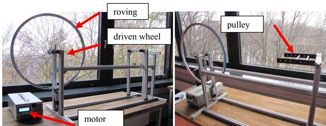
**Figure 1.** Apparatus for simulation of wear of roving
