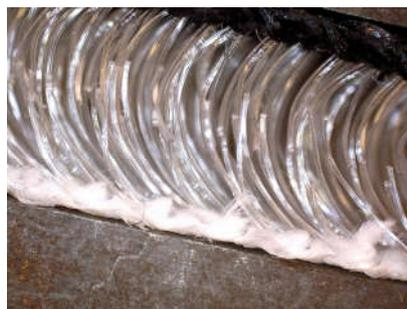
**Figure 1.** View of a 3D spacer fabric from the side.
