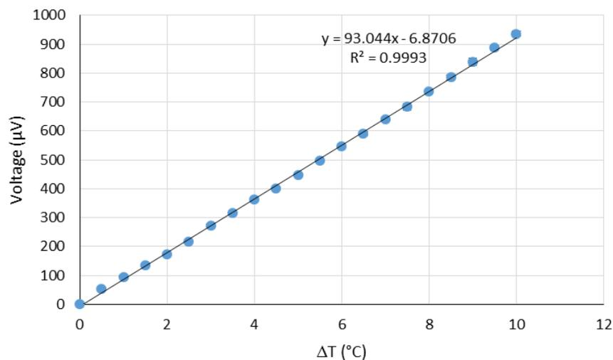
**Figure 3.** Graph of voltage versus temperature difference from 36-pair CF-NiCF junction after the etching process.
